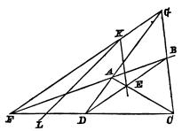
Then E is the pole of FG, and if the given tangent KL meet FG in K, E is on the polar of K; therefore the other tangent through K forms an harmonic pencil with KF, KL, KE.
